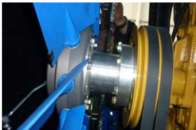
Reversible Fan - recommended for dusty applications
